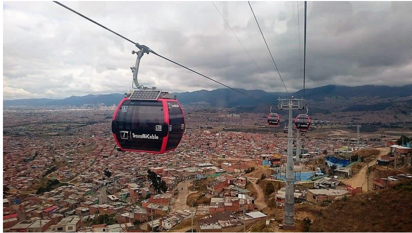
Figure 7: Solar powered gondola in Bogota slum
