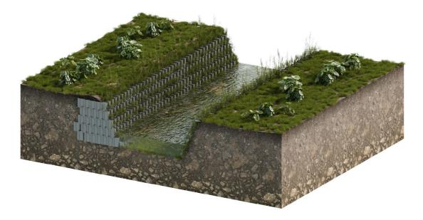
Figure 69 Structural geocell containment in embankment (Source: Guajava, 2023).
