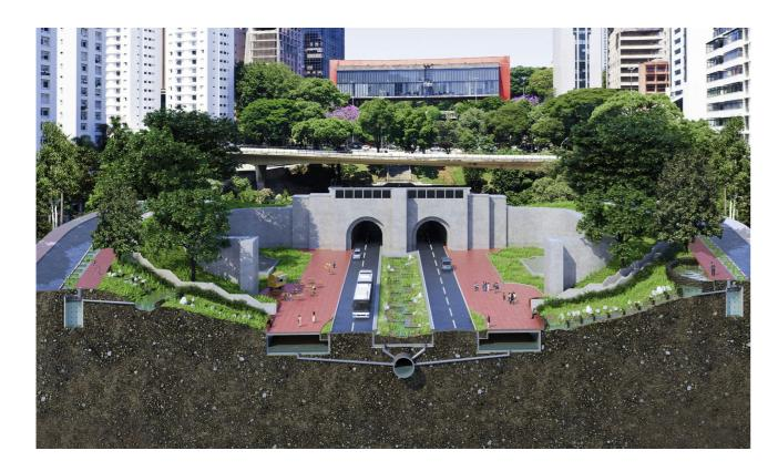
Figure 73 Project cross-section, highlighting the proposal of a new NbS: rain terrace (Source: Prefeitura de São Paulo, FCTH, 2021).
