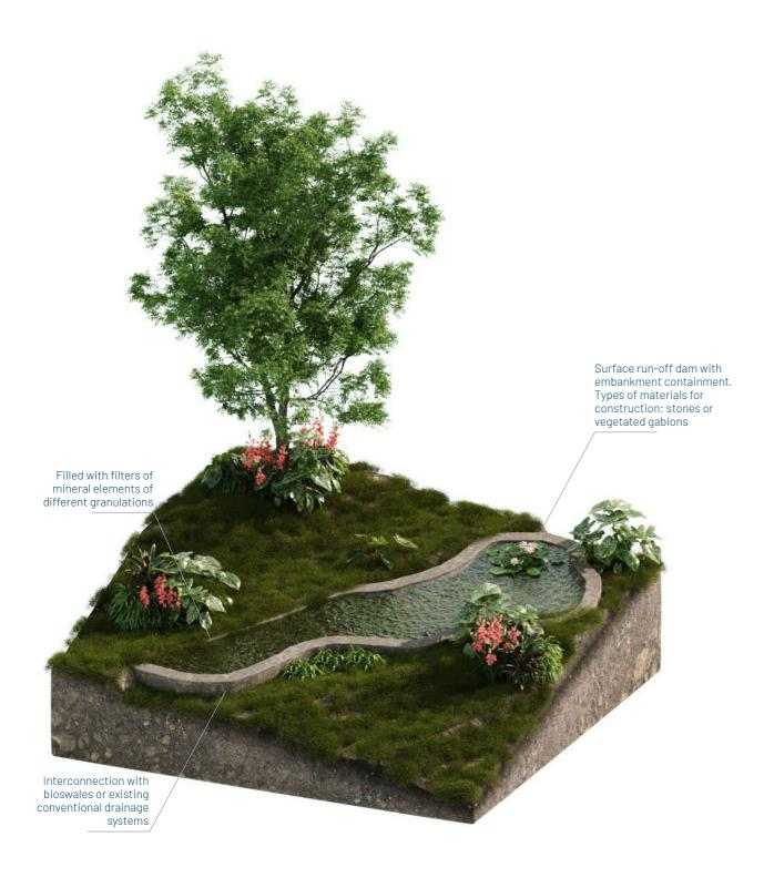
Figure 15 Rain terrace on embankments (Source: Guajava, 2023).
