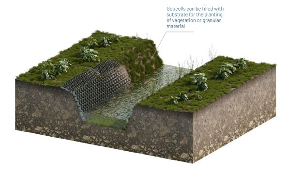
Figure 68 Surface geocell containment in embankment (Source: Guajava, 2023).
