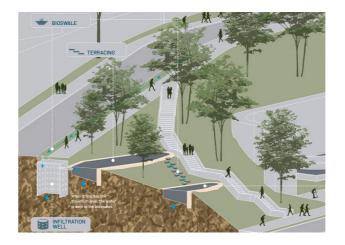
Figure 75 Saracura Infiltration Area showing the location of the NbS: bioswales, rain terraces, infiltration pits, rain bed and underground reservoir.
