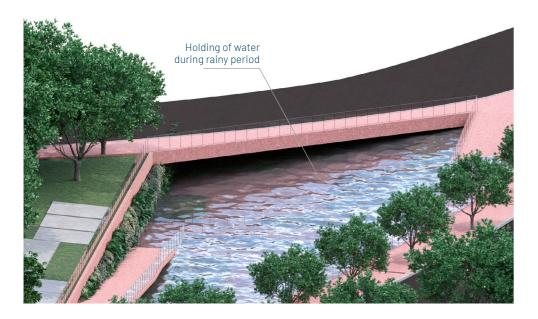
Figure 40 Full amphibious reservoir, internal view (Source: FCTH, 2021).
