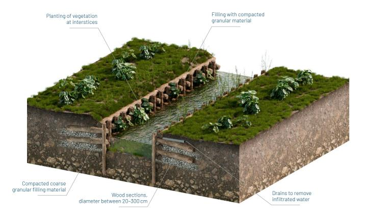
Figure 51 Riverbank cribwall (Source: Guajava. Adapted from Helgard, Z., 2007).
