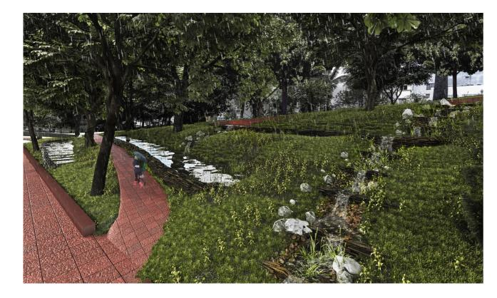
Figure 74 Perspective of the NbS, focusing on the rain terrace and bioswales (Source: Prefeitura de São Paulo, FCTH, 2021).
